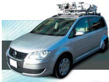
図4 Mobile Mapping System (三菱) [2]
